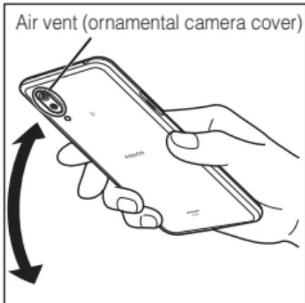
**3 Wipe off water remaining in the grooves of each section by gently putting the product against a dry and clean cloth etc.**
